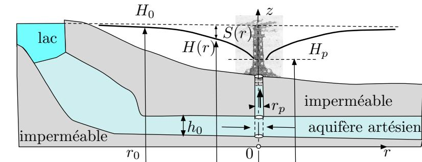
$$S(r) = H_0 - H(r) = \frac{Q}{2\pi T} \ln \left( \frac{r_0}{r} \right) \quad \text{avec} \quad T = K_p h_0$$
