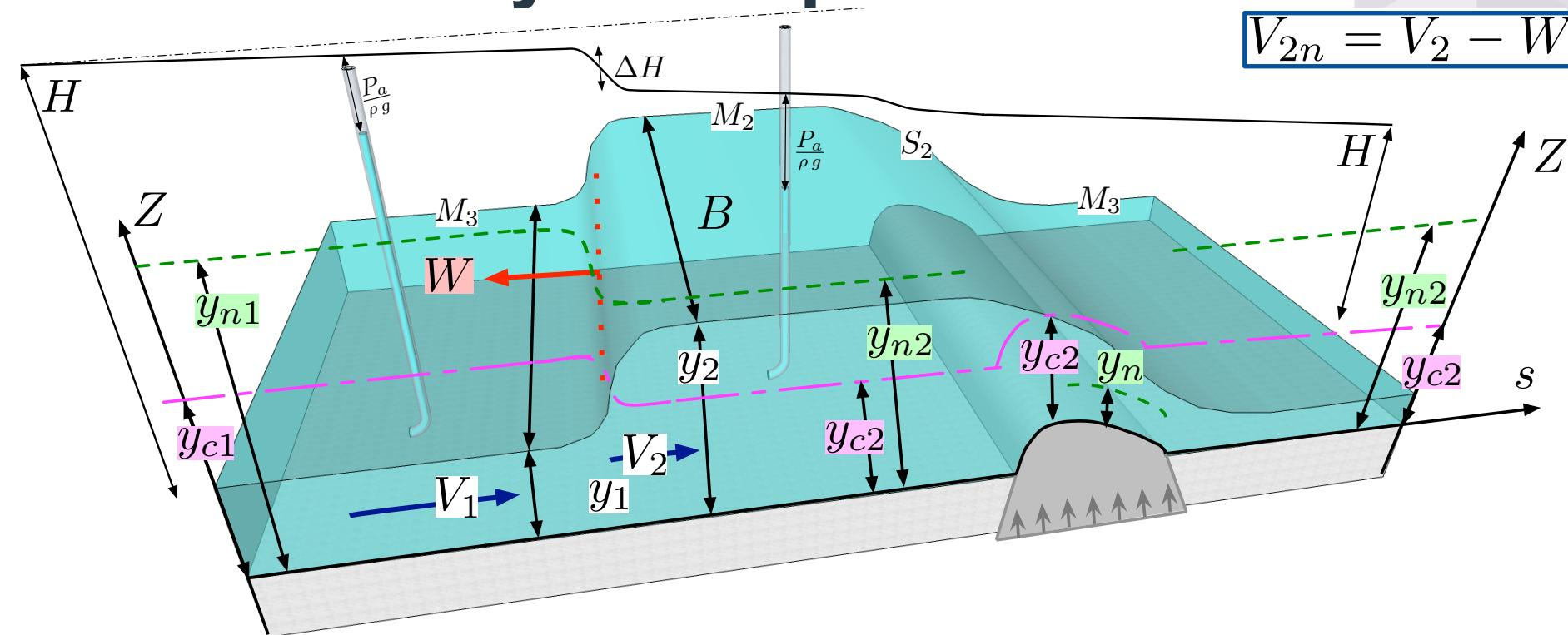
$$y_1 V_{1n} = y_2 V_{2n} \quad \text{et} \quad y_1 V_{1n}^2 + \frac{1}{2} g y_1^2 = y_2 V_{2n}^2 + \frac{1}{2} g y_2^2 \implies$$
